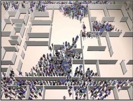
Figure 11: Snapshot from a simulation of 1,000 people evacuating an office environment.
